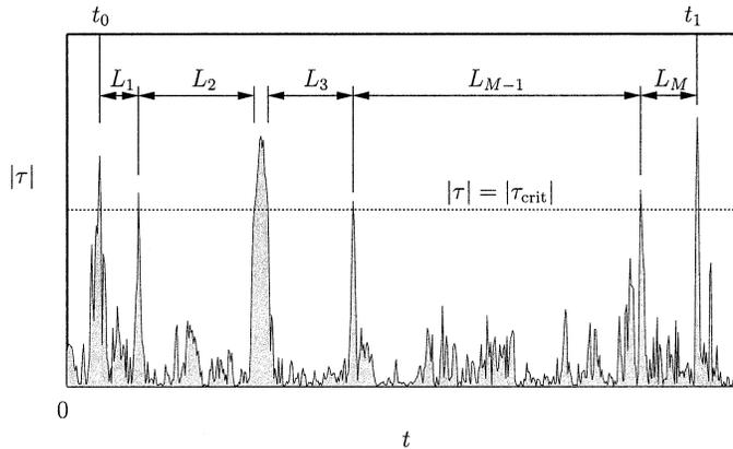
Fig. 4. Representative history of hydrodynamic stress magnitude showing the division of the record into stress lulls,  $L_1$ ,  $L_2$ , etc., for a given value of the critical stress,  $\tau_{\text{crit}}$ .
