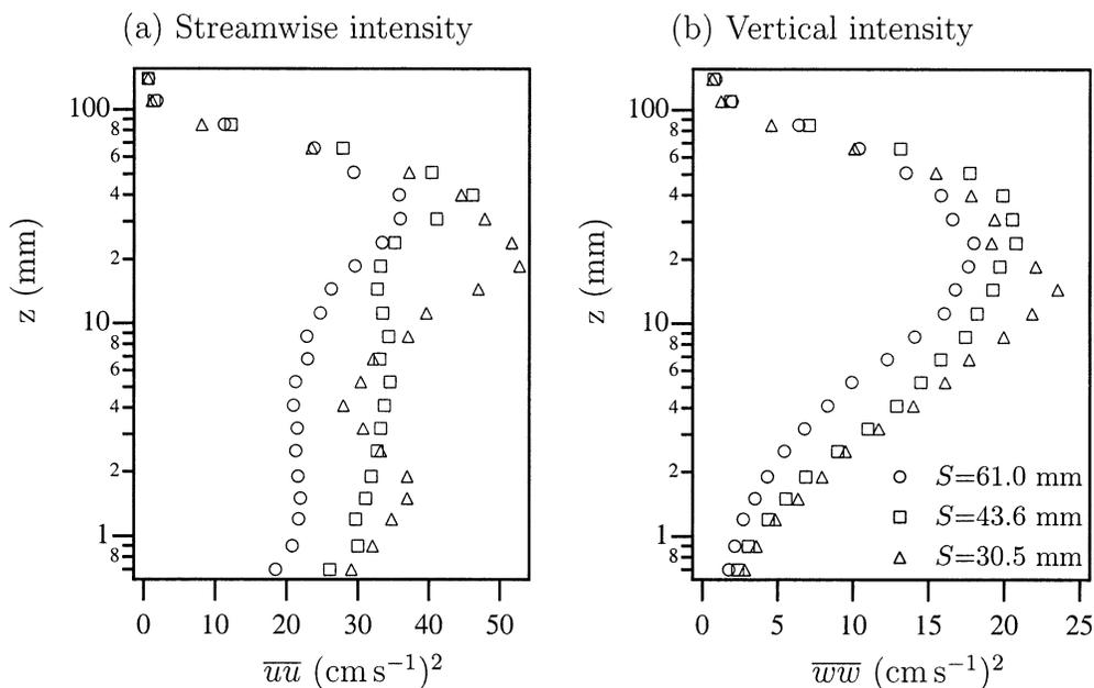
Fig. 6. Effect of adult clam spacing on (a) streamwise and (b) vertical turbulence intensity profiles for  $U_\infty = 40 \text{ cm s}^{-1}$  and  $h = 18 \text{ mm}$ . Values of the adult clam spacing  $S$  are shown above.
