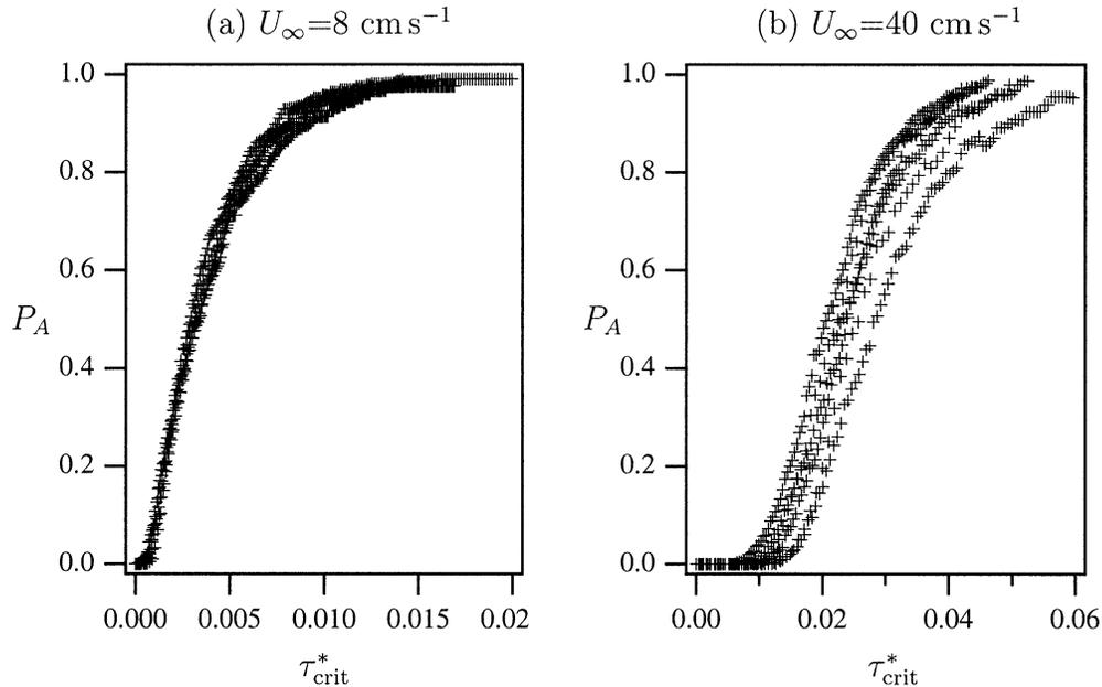
Fig. 11. Anchoring success probability for all experimental conditions versus the nondimensional stress parameter  $\tau_{\text{crit}}^*$  with  $t_a = 4$  s. Results are shown for (a)  $U_\infty = 8 \text{ cm s}^{-1}$  and (b)  $U_\infty = 40 \text{ cm s}^{-1}$ .
