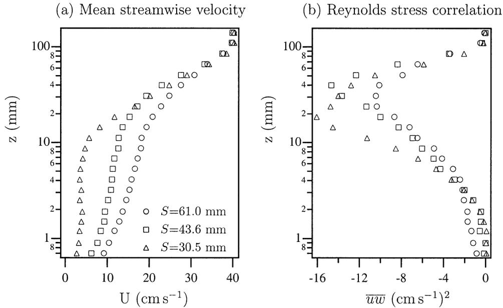
Fig. 5. Effect of adult clam spacing on (a) streamwise velocity and (b) Reynolds stress correlation profiles for  $U_\infty = 40 \text{ cm s}^{-1}$  and  $h = 18 \text{ mm}$ . Values of the adult clam spacing  $S$  are shown above.
